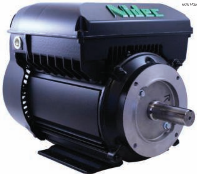
FIGURE 3. This 3–10 hp electronically commutated motor with an IE4 rating integrated with a tuned variable frequency drive is part of the ACCU-Series line of variable speed products. The brushless permanent magnet motor and drive have an integrated user interface that allows for easy setup
