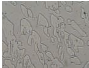
FIGURES 3 AND 4. Proper heat-treatment of metal valve components can have a crucial effect on valve performance. The micrograph on the left shows a non-heat-treated metal structure at 200-times magnification, while the right image shows the metal after heat-treatment (same magnification)
