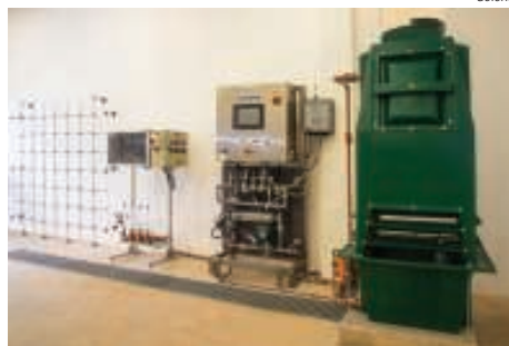
FIGURE 1. Engineers run water-quality models using a cooling-tower pilot plant to determine the effectiveness of treatment chemicals
