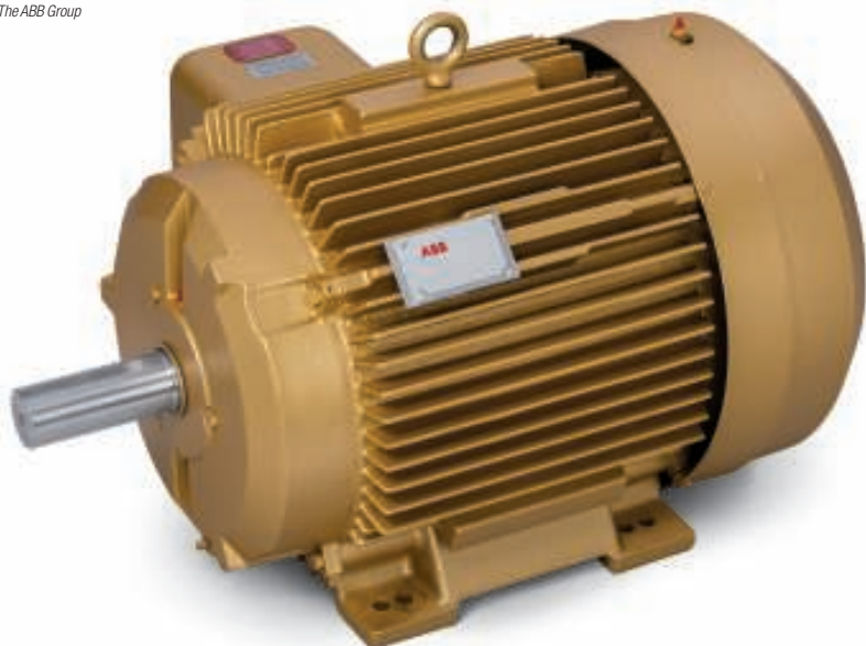
FIGURE 2. The ABB Ability Smart Sensor provides remote condition monitoring for low-voltage motors. It attaches to the frame of the motor, without wires, and picks up data on vibration, temperature and other parameters
