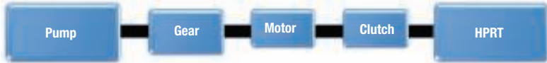
FIGURE 5. Shown here is the arrangement of an HPRT with pump drive at greater than motor speed
